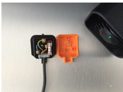
Triple core cable with 0.75mm 2 cable diameter
